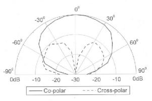
Fig. 7. Radiation pattern of conventional SQMA measured at 8.80 GHz.
