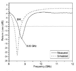
Fig. 4. Variation of return loss versus frequency of SMSA.
