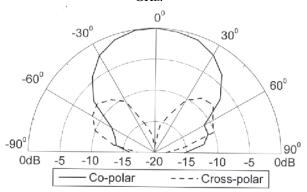
Fig. 8. Radiation pattern of SCSQMA measured at 9.91 GH.
